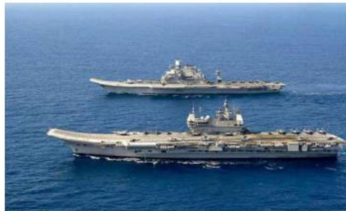
Huge vessel: The INS Vikrant is powered by four General Electric LM2500 engines which give it a maximum speed of 28 knots and an endurance of 7,500 nautical miles. PTI
